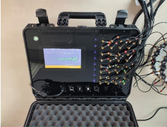
As shown in Figure 2, the system consists of eight four-channel measurement cards connected via an FD CAN bus to a measurement module. With a sampling rate of up to 4MBPS, each channel has its generator of alternating square waves with amplitudes of up to 144Vp-p and a maximum current capacity of 3A at any given time. Each channel has three eight-order filters, as shown in Figure 3, which display a measurement card with shielding capabilities.
