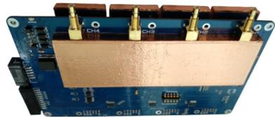
Figure 4 illustrates an analog module with an integrated amplifier, AD8331, with gain control via an external DAC converter, a signal conversion system for alternating acoustic signals to envelope ADL5511, and two differential amplifiers, THS4521.
