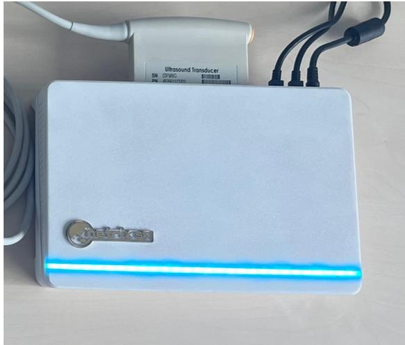
The device uses two measurement techniques that are complementary to each other: ultrasonic tomography and electrical impedance tomography. The complementarity of these techniques is that EIT has high resolution at the edge of the measurement area, while UST performs better inside it. Therefore, the fusion of these two techniques is expected to produce an image with a much better resolution than relying on only one of them.
