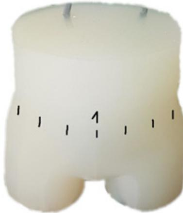
For the reflection method, electrodes were applied to each point in turn, i.e., signal measurement was performed using ultrasonic transducers with different frequencies. The circumference of the phantom at the places where the electrodes are applied was 38 cm. The number of electrodes was 19. A mesh was made for the cross-section of the phantom at the electrode locations (Figure 2). Additionally, the electrodes were marked. There were 548 nodes and 999 finite elements.
