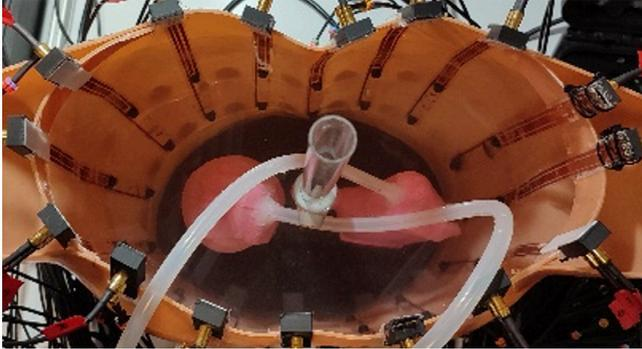
Graphite electrodes with a diameter of 4 mm were attached to the phantom, placed on laminated copper tapes, and secured with plastic sleeves. These electrodes are connected to PCBs that contain SMB sockets and mounted on the aforementioned tapes. Each electrode is part of a complete mounting system, which allows easy placement around the phantom circuit.
