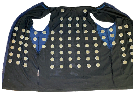
Figure 1. The inner part of the vest. The electrodes and their location are visible
