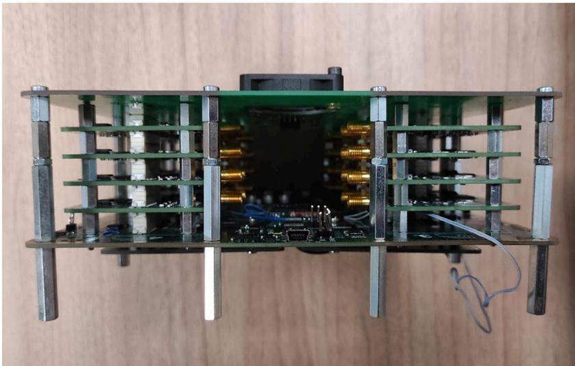
The following Figure 2 shows the assembled measuring cards. And Figure 3 shows the tomograph folded into its housing. The tomograph is equipped with a rechargeable battery, which allows it to operate autonomously, independent of a power source.
