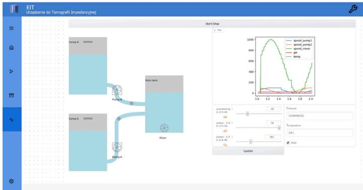
During dosing, process parameters such as pH and temperature are measured, and a reconstruction is made from the tomographic measurements (reconstructions can be observed in another tab of the application). In turn, the unit controls the feeding of the two substrates and the mixer in the main tank.
